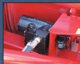
HYDRAULIC MOTOR DRUM ROTATION WITH GEAR AND CUSHION VALVE
