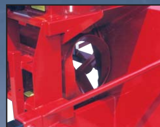
REMOVABLE ROTARY DRUM WITH TWO POLYETHYLENE BEARINGS (FRONT AND BACK) FOR EASY MAINTENANCE
