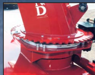
CHUTE ROTATION ON POLYETHYLENE UHMW TO AVOID FRICTION AND ICE ACCUMULATION
