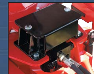
HYDRAULIC CHUTE ROTATION WITH GEARS, MOTOR AND CUSHION VALVE
